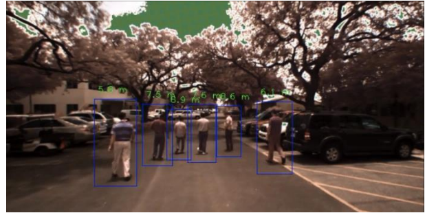
Figure 8. SwRI's Image-based Pedestrian Detection
